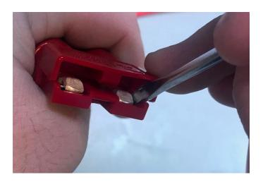
Once the tongue is depressed, gently pull the contact out of the housing by giving a light tug on the wire.
