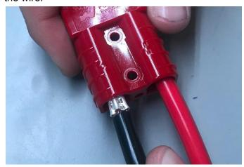
If it won't come out with a light tug, place the screwdriver below the contact to allow it to pass over the tongue as shown below:
