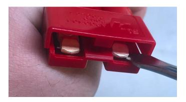
Once you have removed the cable from both sides, take the appropriate wire, and with the SB50 firmly on a table or similar hard surface, push on the back of the contact so that the tab snaps back over the tongue.
